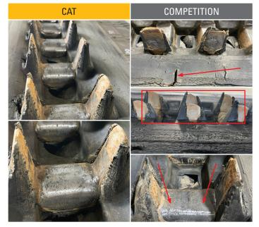
The competition exhibited several wear patterns that led to detracking and vibration issues, while the Cat tracks stayed within acceptable wear limits. These wear patterns can cause reduced lower productivity and operator comfort, while also limiting the service life of the track. Improper engagement with the sprocket can also lead to premature wear of that component, increasing undercarriage maintenance costs for the customer.
